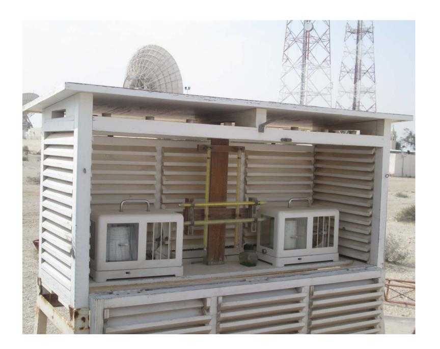
Also measurements for Relative humidity and dewpoint are carried out by dry and wet bulb thermometer, Lambrecht hygrograph and in AWS Vaisala sensors.
